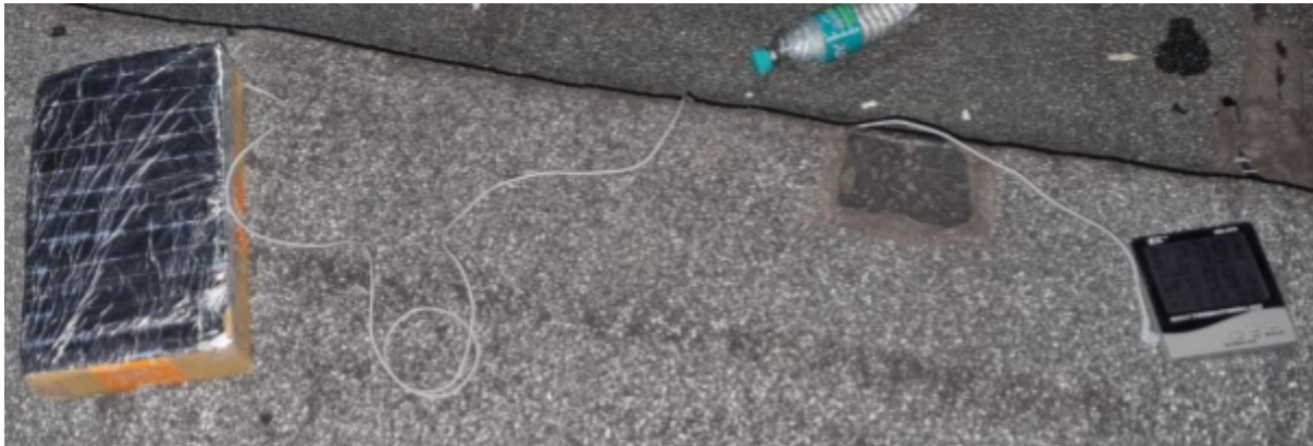
Test setup of the experiment conducted at night. The device on right is the temperature sensor.
