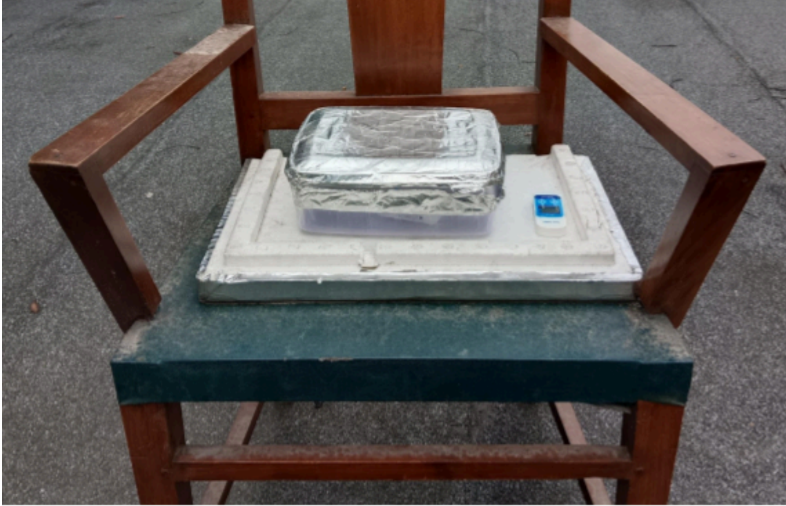
Test setup of the experiment. The plastic box, covered with reflective material. Data loggers are used in this experiment.
