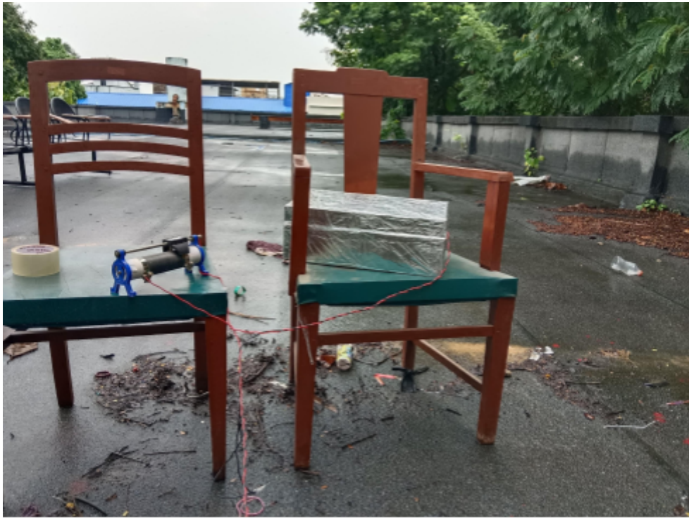
Test Setup of the experiment. Rheostat is used to vary the heat loads.
